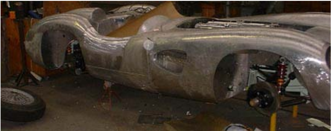
The aluminium body of Les Johnson's Aston Martin DB R takes shape
